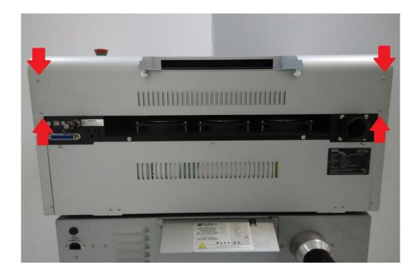
4. After the back cover is removed, you can reach the power board assembly (red squared) on the left.
