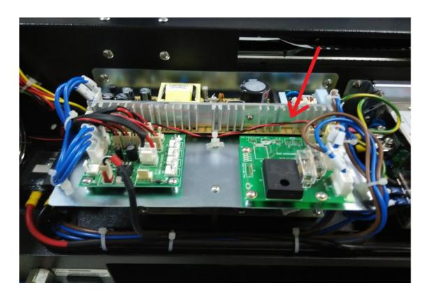
6. Refer to below picture and unplug all cables on the 12V transfer board.
