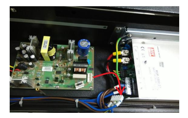
9. Then, loosen the four screws which fix this power board, then we can remove the board, we will replace this board with new power supply.
