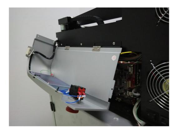
5. Loosen the four screws on the protection cover. (no need to remove the one with ground cable connected)
