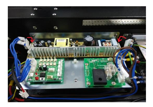
21. Restore all the 2-pin cables to 12V converter board (each cable can plug into any slot on the converter board, they are all the same except the bottom one with red circle, it needs to be plug into its specific slot)
